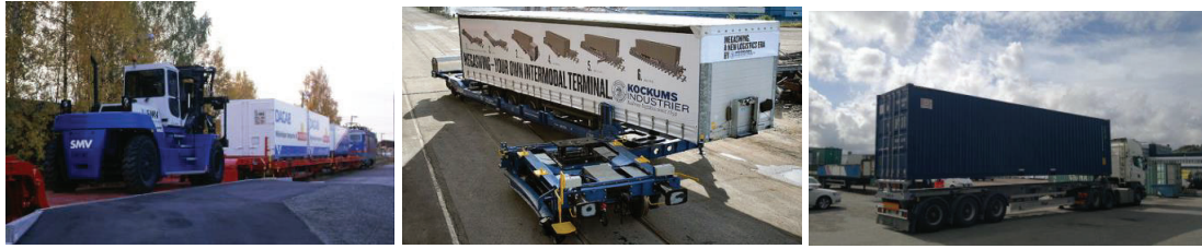
Figure 4 Examples of novel transshipment technologies from left: The Light-Combi System; Megaswing and ACT.
