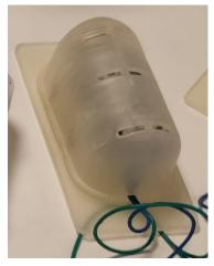
Figure 18: Haptic motor for the seat
