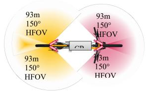
Figure 11: Radar mounting configuration in the prototype
