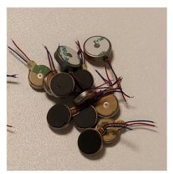
Figure 19: Haptic motors for handlebar
