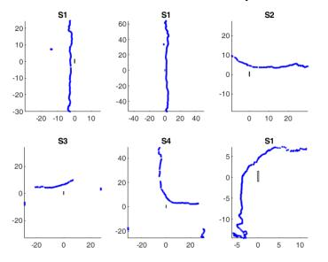
Figure 14: Tracked relative trajectories of approaching vehicles, different scenarios
