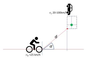
Figure 10: Front collision use cases (left, right)
