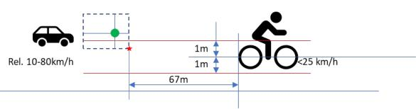
Figure 8 Rear closing vehicle use case
