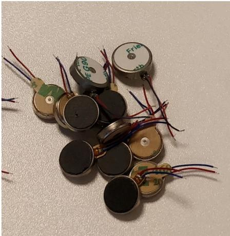
Figure 19: Haptic motors for handlebar
