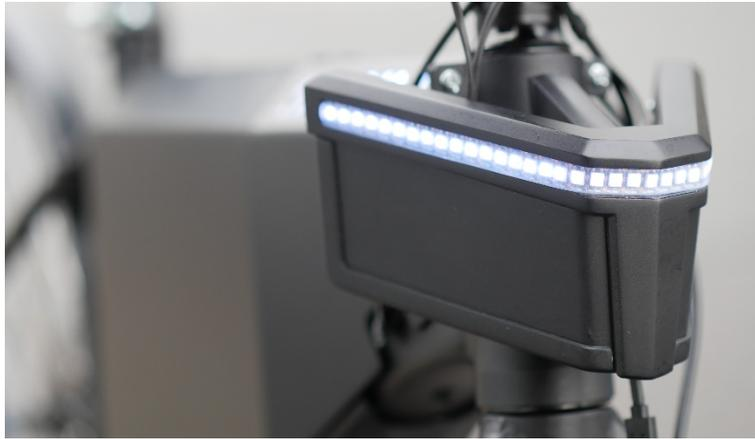
Figure 20: Front LED warning light
