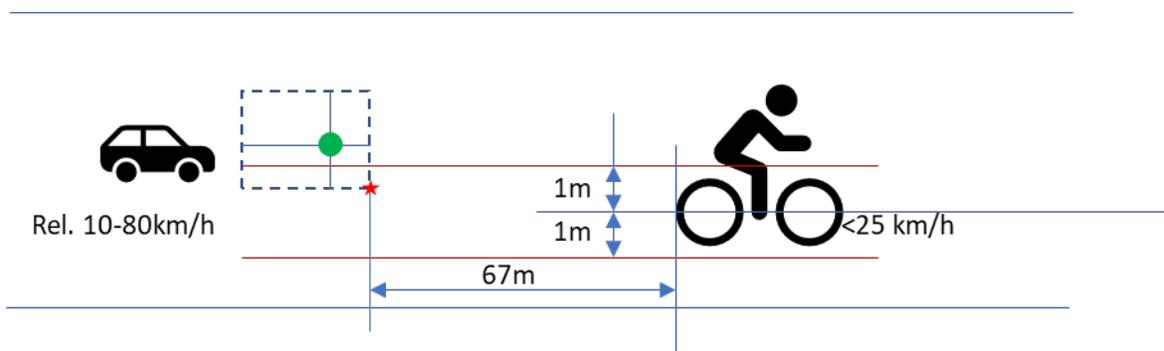
Figure 8 Rear closing vehicle use case
