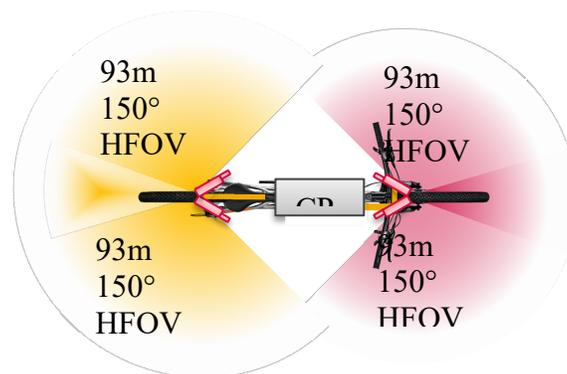
Figure 11: Radar mounting configuration in the prototype
