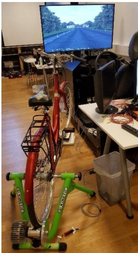
**Figure 17: Bicycle simulator in Victalab (with other testbike)**
