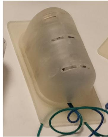
Figure 18: Haptic motor for the seat
