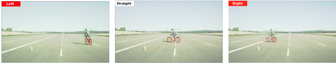
Figure 6: Bicycle orientation estimation based on the proposed ellipse detector and a simple decision tree.
