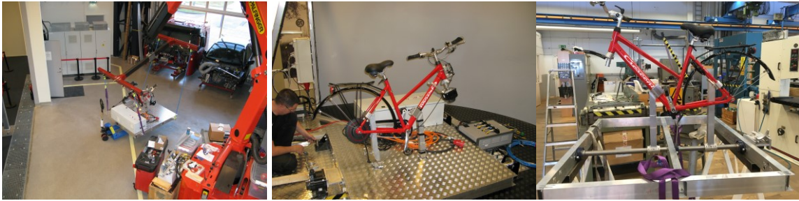
FIGURE 1 Constriction of the platform, the entire system attached to a crane (left), the system mounted to the simulator (middle) and the aluminum construction of the base with the bicycle on top (right).
