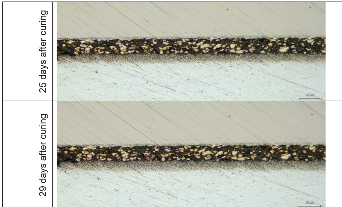
Figure 7 Light optical microscopy results of cross-sections at 200x magnification a few hours after curing, 7 days after curing, 15 days after curing, 25 days after curing and 29 days after curing.
