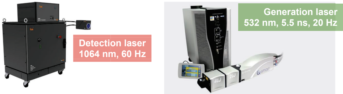
Figure 3: Photos of (left) the detection laser system, and (right) the generation laser system of the high power (HP) measurement system.
