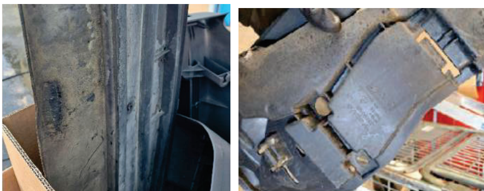
Figure 23. PP plastic with EPDM and mineral filler, from 20-year-old V70 and V50.
