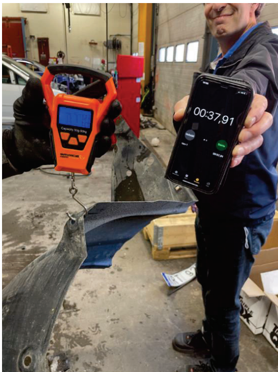
Figure 3. Plastic weight, dismantling and cleaning time was measured.
