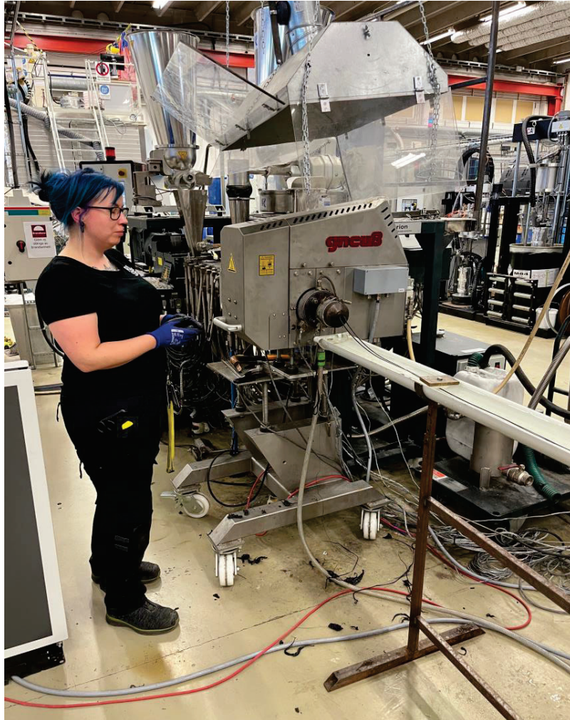
Figure 26. Compounding in a Coperion ZSK 26 twin-screw extruder equipped with a Gneuss melt-filter system.
