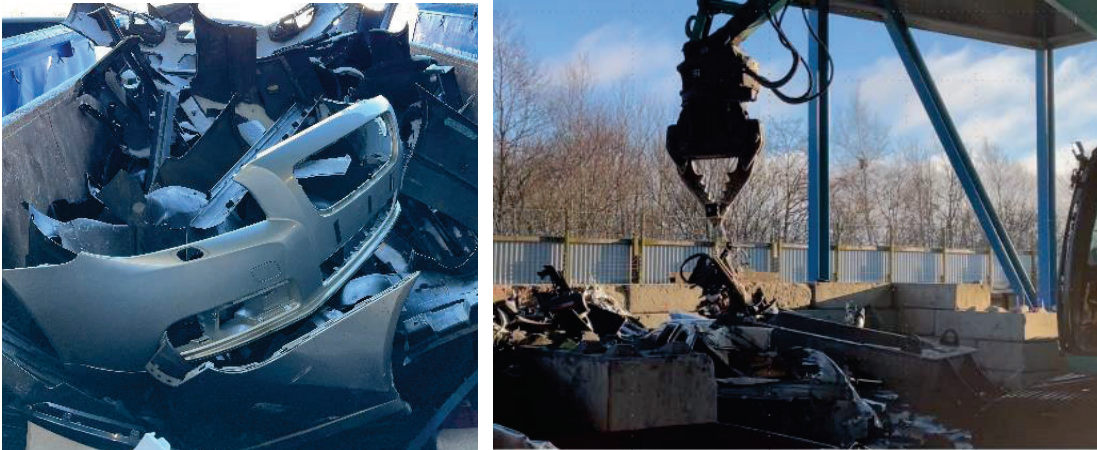
Figure 2. Examples from site visits and handling practices. Jönköpings Bildemontering has started to sort out parts of PP plastic. Eklunds and Walters dismantle the cable harnesses using a power grip.
