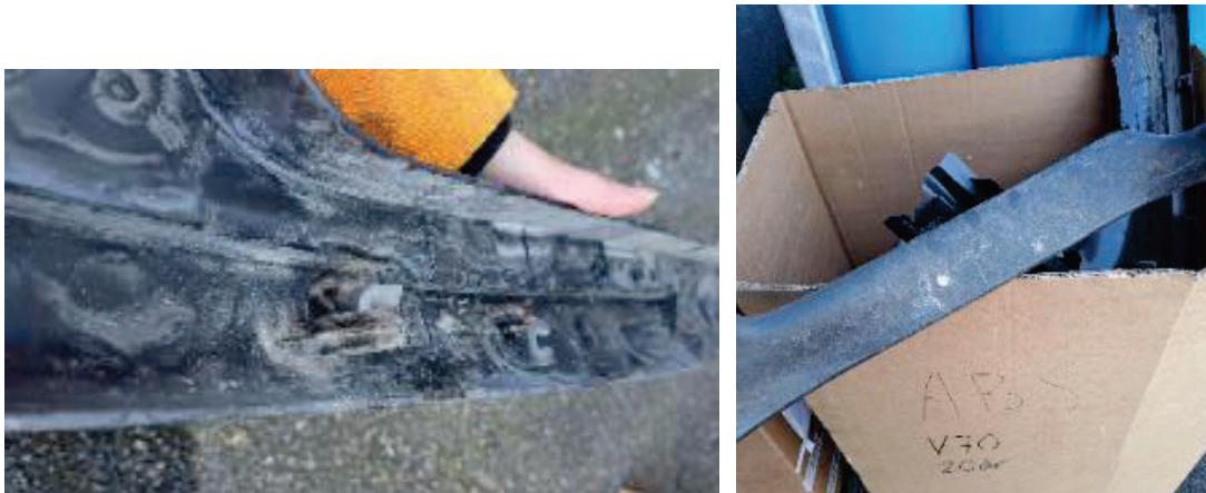
Figure 22. ABS from 20-year-old V70 and V50.
