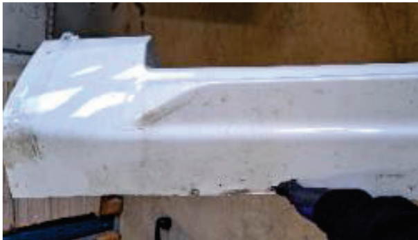
Figure 25. Painted PP with EPDM, from 10-year-old XC90.
