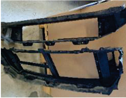
Figure 24. PP with glass fibre, from 10-year-old XC90.
