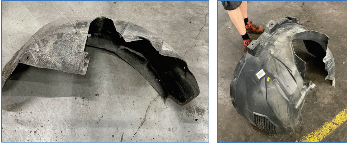
Figure 19. Inner fenders made of PET and PP-based material respectively.
