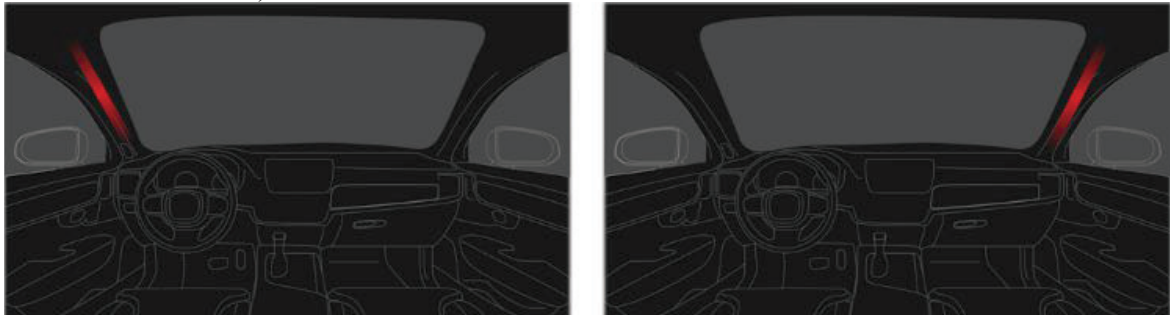
Figure 3: Illustration of the location and shape of ambient light that showed the approach or breach of the lane line or lane edge.
