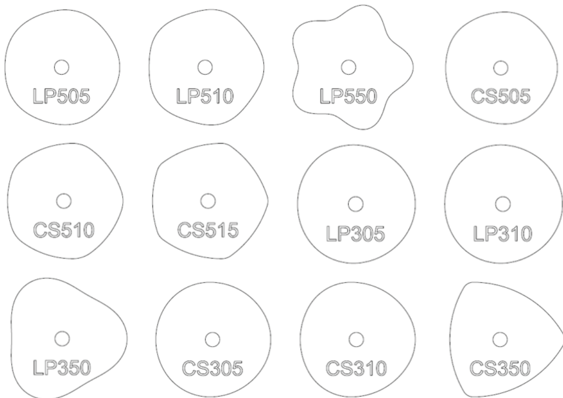
Figure 2- Test specimen for measure method uncertainty evaluation
