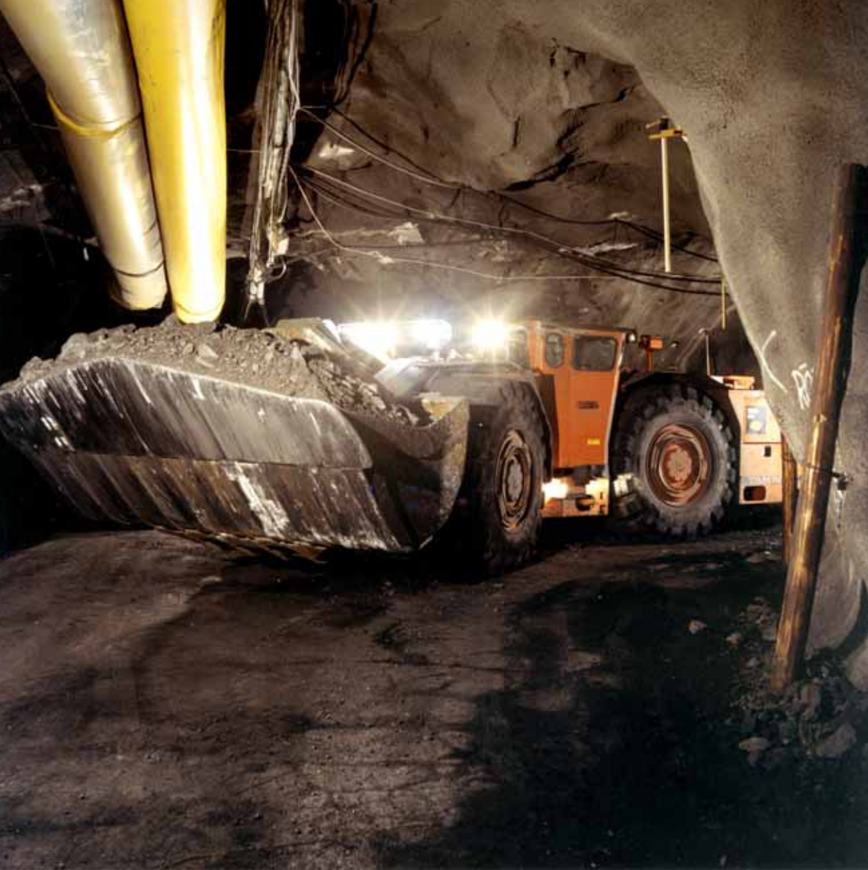
A bucket loader moving excavated ore in the mine. (Image: LKAB).
