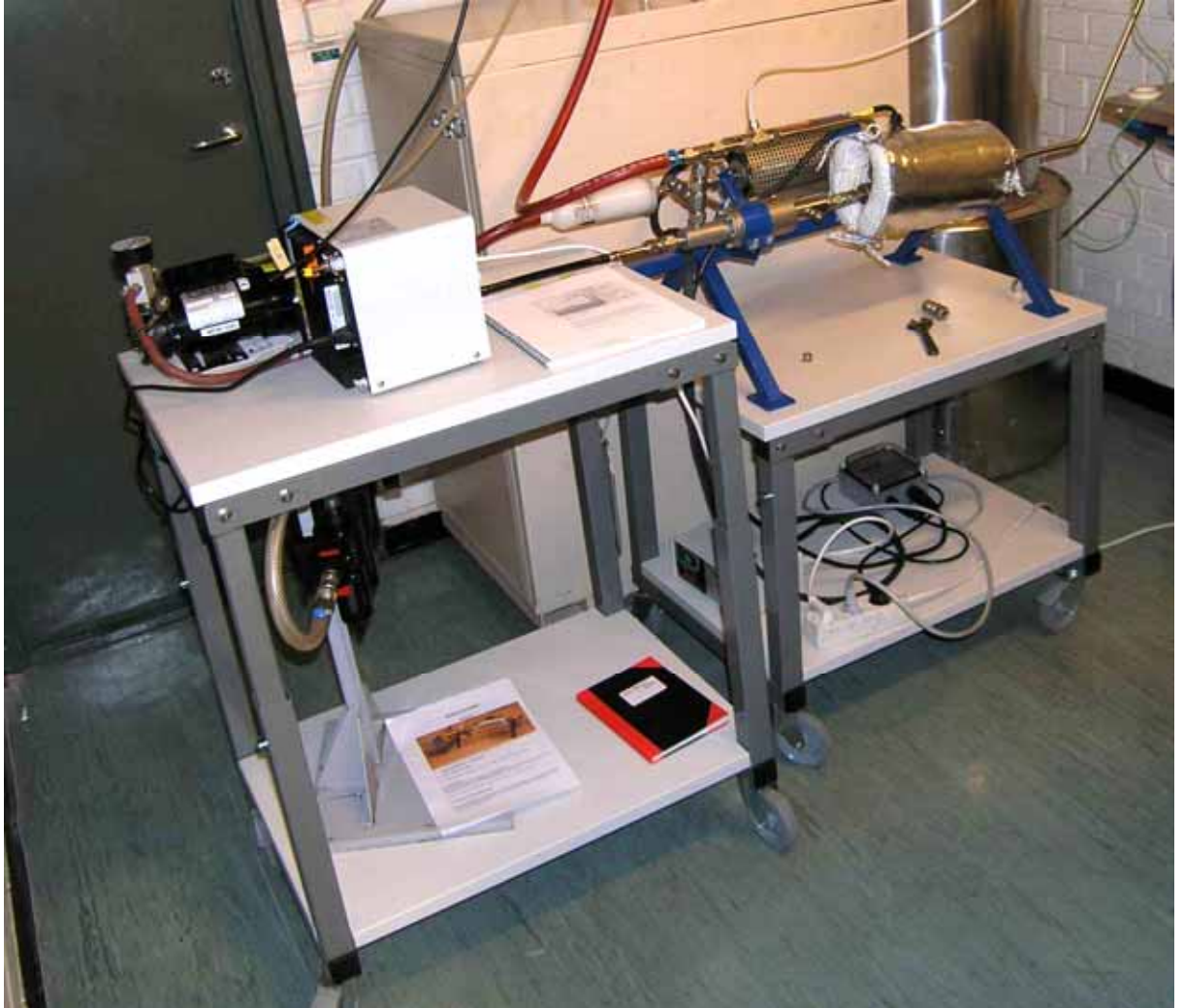
Figure 10 The basic setup of the measurement system with two diluters
