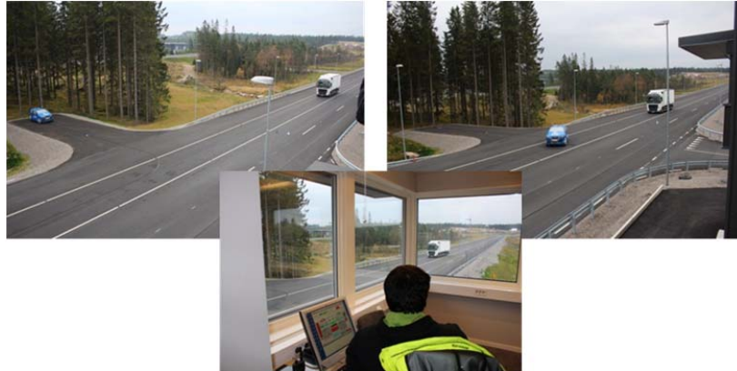
Figure 6 – Automated testing on the test track. Cut-in scenario where the truck approaches an intersection where the balloon car suddenly drives out in front of the truck. Truck and balloon car driven by robots. Complete scenario controlled from the control room. (AstaZero Multilane test track).
