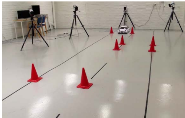
Figure 7 – Photo of the scaled test track for the double lane change demonstration. There are two lanes in the track, defined by the red cones shown in the picture.
