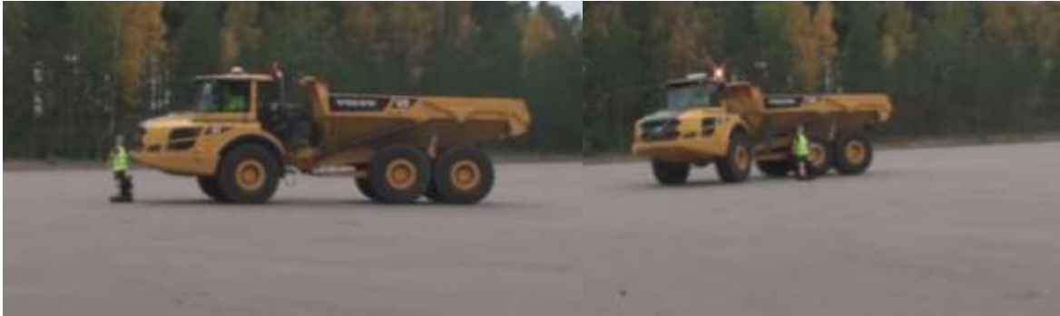
Figure 5: Pictures from the movie recorded during the demonstration of automatic emergency braking in Eskilstuna, 2014. The picture to the left shows a close call when the machine has stopped just before hitting the dummy. The picture to the right shows how the machine can drive around close to the dummy without the algorithm generating any false intervention.
