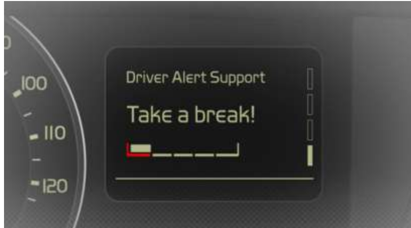
Figure 2: Driver Alert Support is an intelligent system that tracks your driving behaviour. If it differs from normal and indicates tiredness, you are alerted by a signal and a message in the display, advising you to take a break
