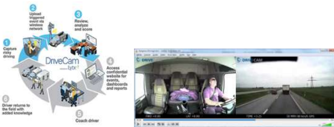
Figure 3: Overview of the drivacam program plus an Example of the video event recorder. Note that noise has been added to the driver image due to integrity reasons.
