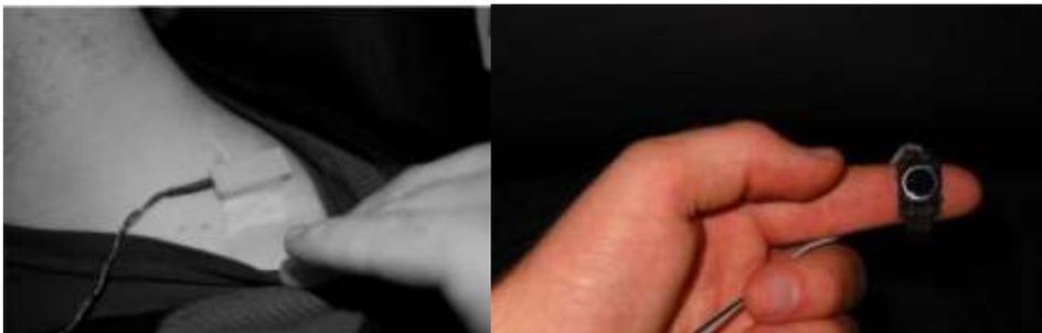
Figure 5 The Tactile DRT factor (left) and response button (right). The basic idea behind the tactile DRT is to measure the cognitive load of an in-vehicle HMI in terms of the ability to respond to tactile stimuli (vibrations) generated by the actor.
