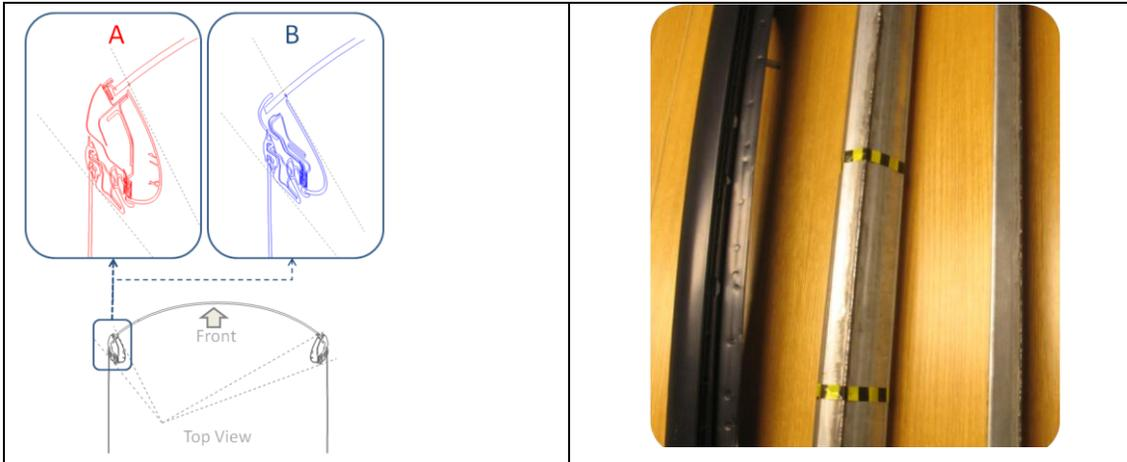
Figure 5. Obscuration angle for State of the Art (A) and folded expandable A-pillar (B) (left picture), and Reference, Expanded and Folded A-pillar (right picture)
