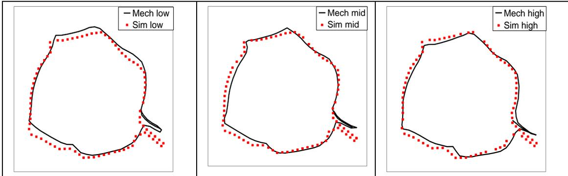
Figure 12. Mechanical and Mathematical Expanded A-pillar Cross Section at  $\frac{1}{4}$ ,  $\frac{1}{2}$  and  $\frac{3}{4}$  of the Length of the A-pillar
