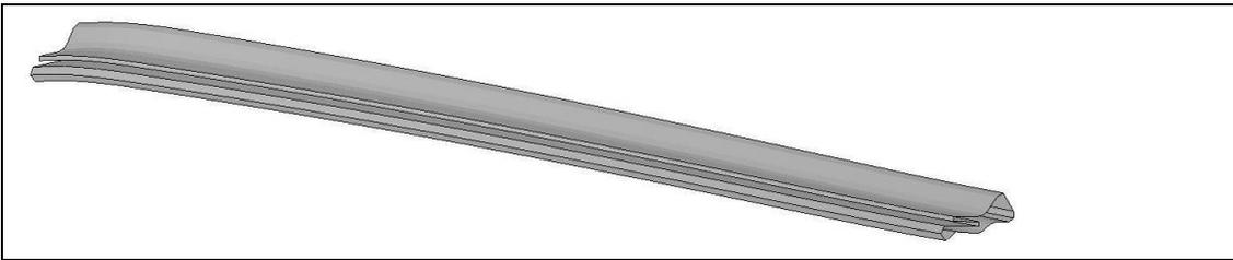
Figure 4. Inflatable A-pillar
