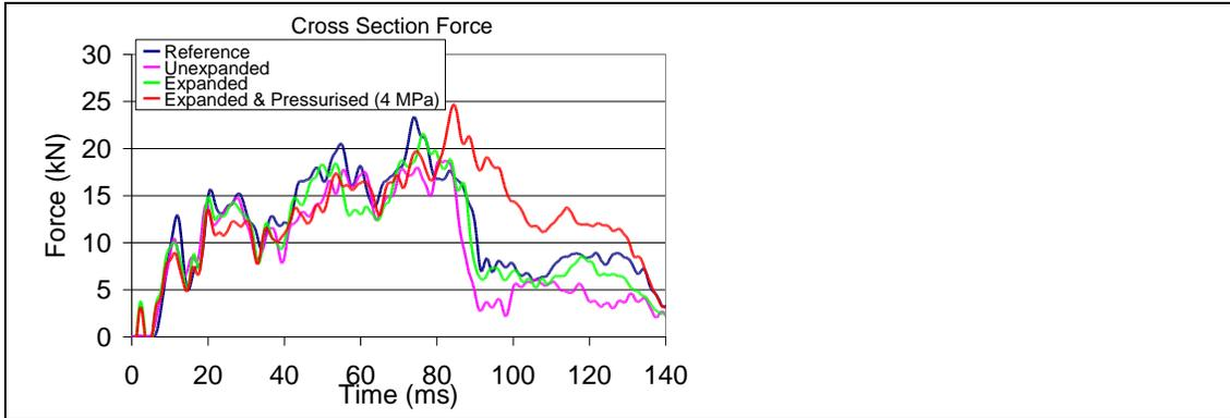
Figure 8. Cross Section Cant Rail Force in Offset Deformable Barrier Crash at 64 km/h (40 mph)
