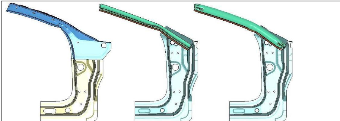
Figure 9. Reference A-pillar, Folded & Expanded A-pillar at 100 mm Roof Crush Displacement
