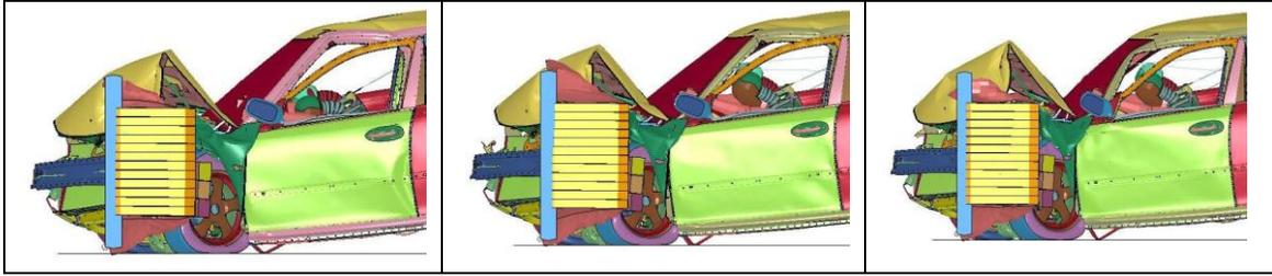
Figure 7. Reference, Expanded and Unexpanded A-pillar at 120 ms in Offset Deformable Barrier Crash Configuration at 64 km/h (40 mph)
