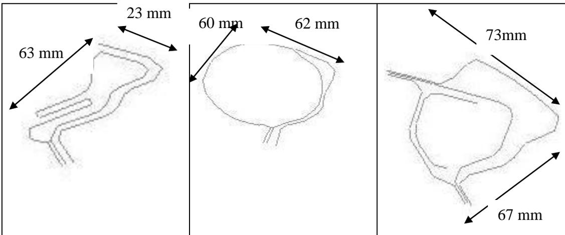
Figure 6. Cross Section of Folded and Expanded Inflatable A-pillar and Reference A-pillar
