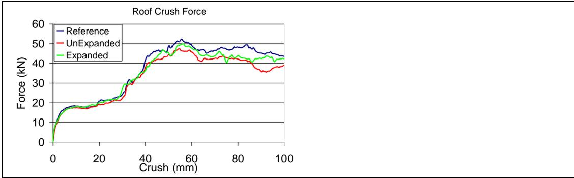
Figure 10. Force vs. Crush for Roof Crush Evaluation
