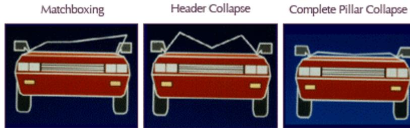
Figure 1. Various Types of Roof Crush
