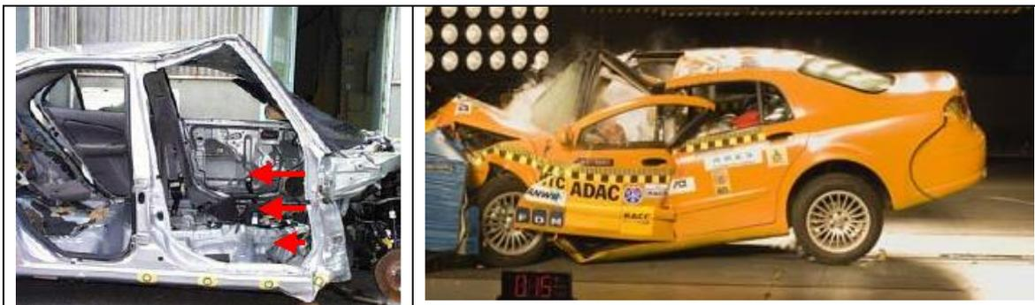
Figure 2. Offset Collisions Exposes the A-pillar to Extreme Loading Conditions [6] and [7]
