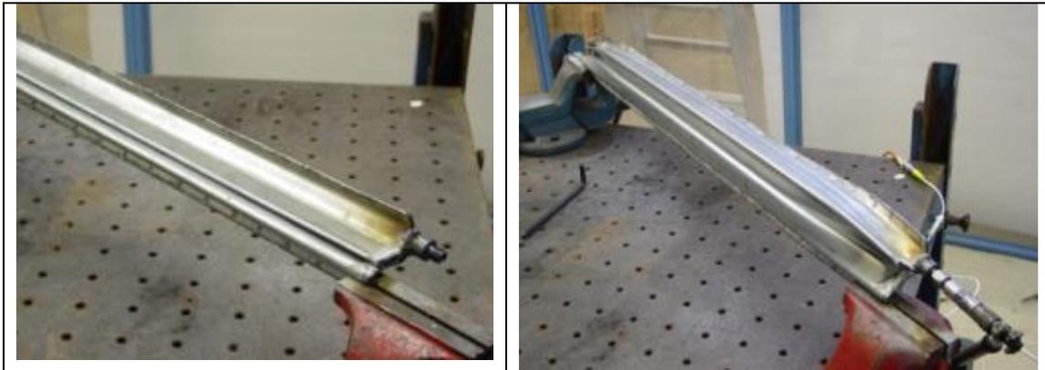
Figure 11. Folded and Expanded Mechanical Inflatable A-pillar Prototype
