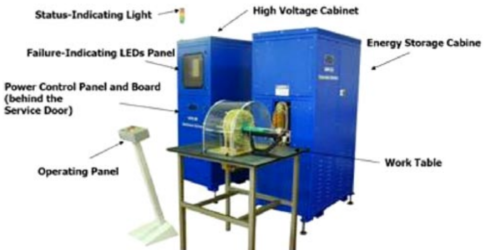
Figure 1 A electromagnetic pulse system for joining axisymmetrical parts.
