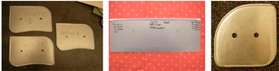
Figure 6 shows on some of the final hemmed parts made by electromagnetic pulse.
