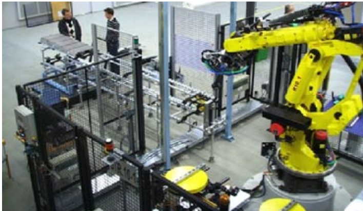
Figure 2. The essential functions of the concept, verified in a test equipment. This includes tugger cart, gravity powered cassettes, car body parts and robot system guided by vision.
