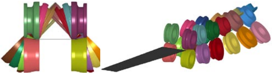
Process set-up for FE simulation of the 3D-roll forming
