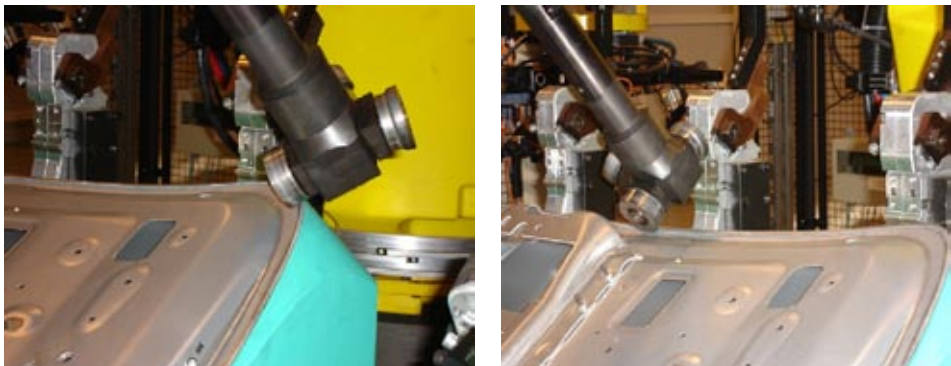
Figure 3 Description of the rollhemming process
