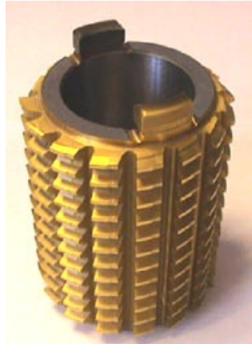
A coated hob for gear cutting
