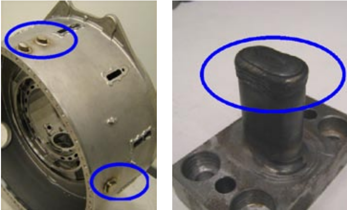
Left: Bosses built on a component with aerospace material
