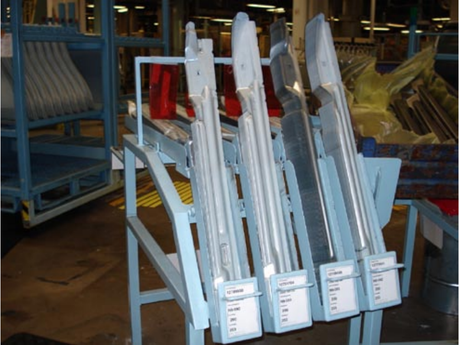
Figure 1: Space efficient minomi presentation of parts at assembly
