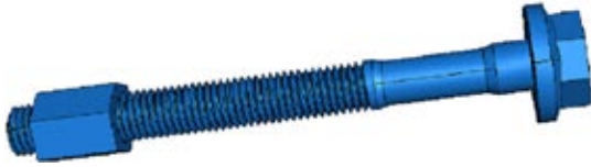
Fig 2 Three-dimensional model of screw joint
